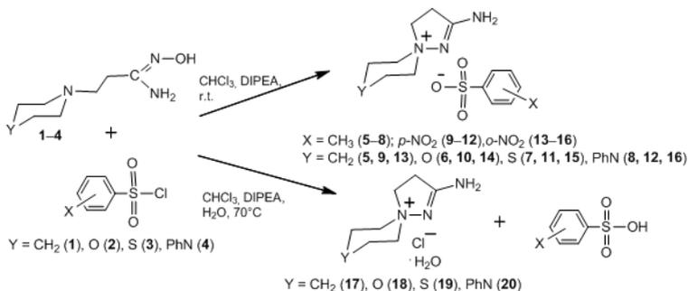
**Scheme 1.** The reactions of tosylation, *para*- and *ortho*-nitrobenzenesulfochlorination of  $\beta$ -aminopropioamidoximes
