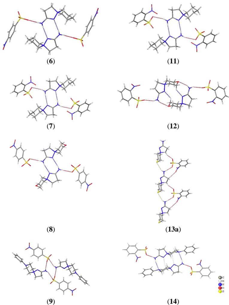
**Figure 4.** H-bonding patterns in crystal structures of studied compounds. H-bonds are depicted with dotted lines
