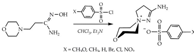
**Scheme 4.** Amينو-4,5-dihydrospiropyrazolylammonium formation at arylsulfochlorination of  $\beta$ -aminopropioamidoximes
